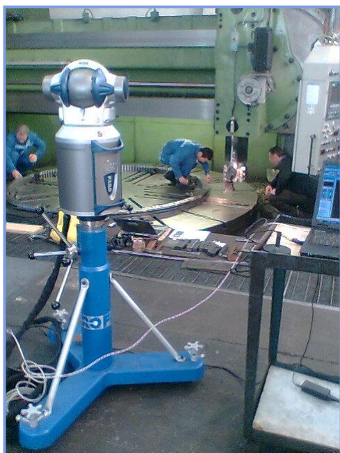
Figure 5 – Measuring the edge of the machine with a laser beacon.
