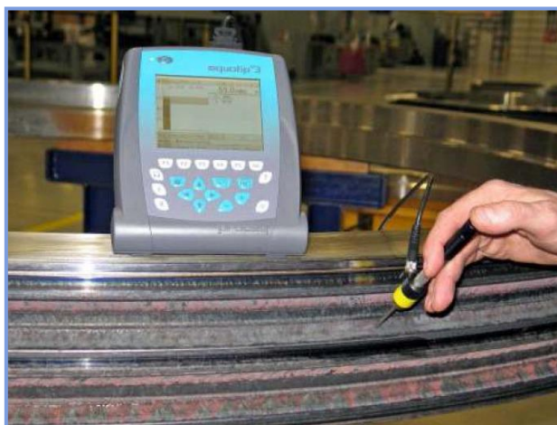
Figure 3 – Race hardness measurement
