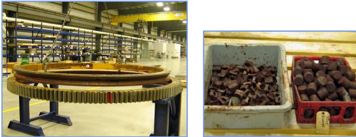
Figure 1 - Crossed-roller slewing bearing with external gear teeth: Rings, rollers and spacers received for repair.
